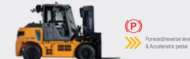
Auto hold: Automatically engages the parking brake when the brake pedal is held for more than 4 seconds.
