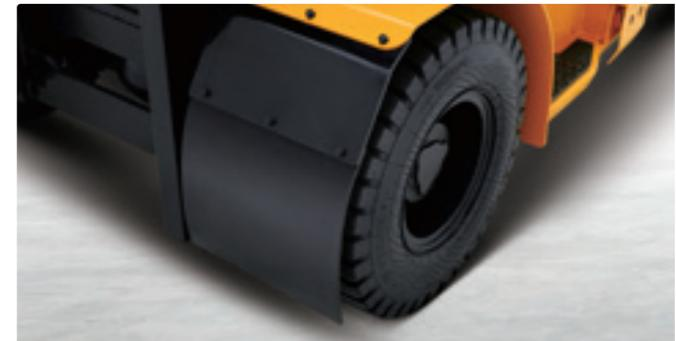
Shields the operator and work environment from debris and contaminants kicked up from the front tires.
