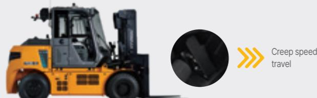
Allows travel at 2.5 km/h without pressing the accelerator
