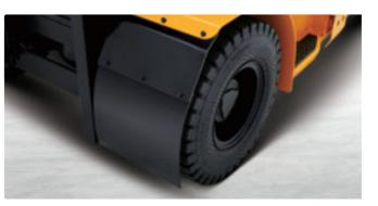
Shields the operator and work environment from debris and contaminants kicked up from the front tires.
