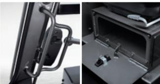
A dedicated mounting bar to the right of the driver's seat and a built-in storage compartment below the cabin help create a personalised and efficient work environment.
