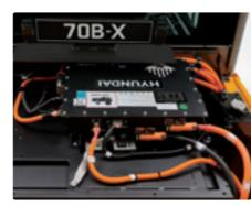
Real-time battery monitoring detects abnormal signals and controls charging/discharging, while activating automatic fire suppression systems as needed to ensure safety.
